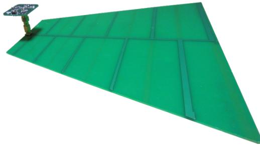
Figure 2.11: The 5-band harvester prototype connected to a log-periodic antenna spanning 400-900 MHz.
