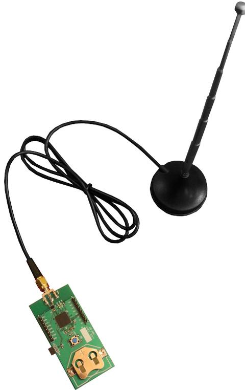
Figure 4.6: Prototype of the wideband ambient backscatter transmitter. The antenna used is a compact, fairly low efficiency monopole designed for reception of TV signals in the 400-900 MHz range. In our experiments this antenna responds sufficiently down to around 100 MHz. The tag itself is composed simply of a TI MSP430F5310, an HMC550A wideband RF switch, and a 20mm coin cell battery.
