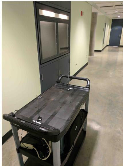
Figure 4.14: Test setup for indoor quality-of-service testing, with antennas separated by 2 ft on a rolling cart.
